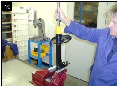
19 Place the cartridge all the way into the strut then lift out to check oil level.
