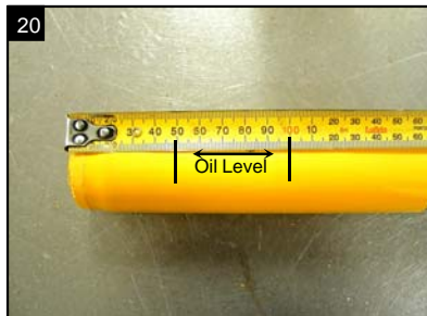
19 Place the cartridge all the way into the strut then lift out to check oil level.
